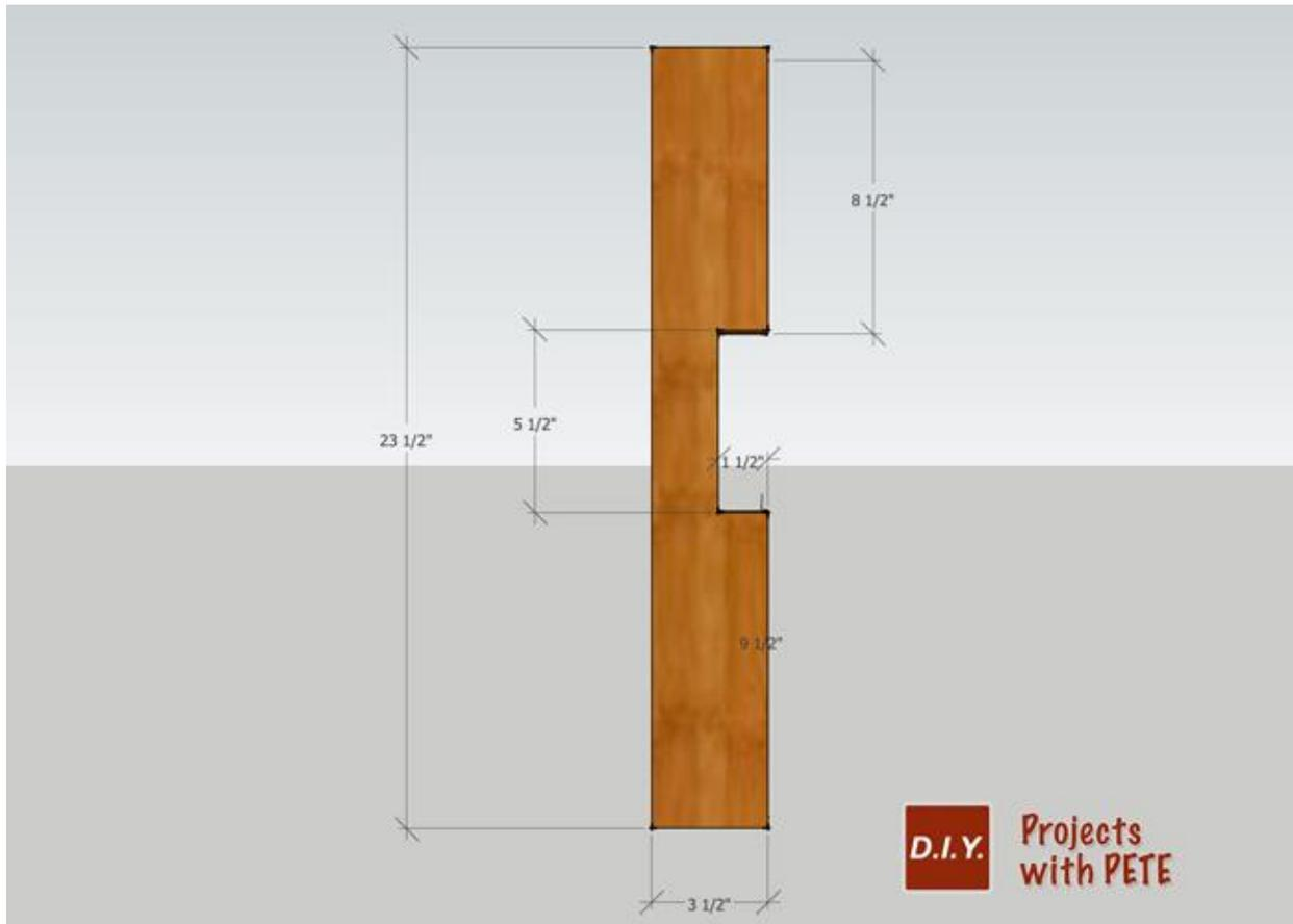
Use a jigsaw to cut out the notch on the two front legs. The 2×6 piece will eventually rest in the notch. Measure 9 1/2 inches up from the bottom of the 2×4 front leg and mark. Measure 1 1/2" back (depth). Then measure from your 9 ½ inch mark up 5.5" and make one more mark. Connect the lines and cut out your notch on both pieces.
