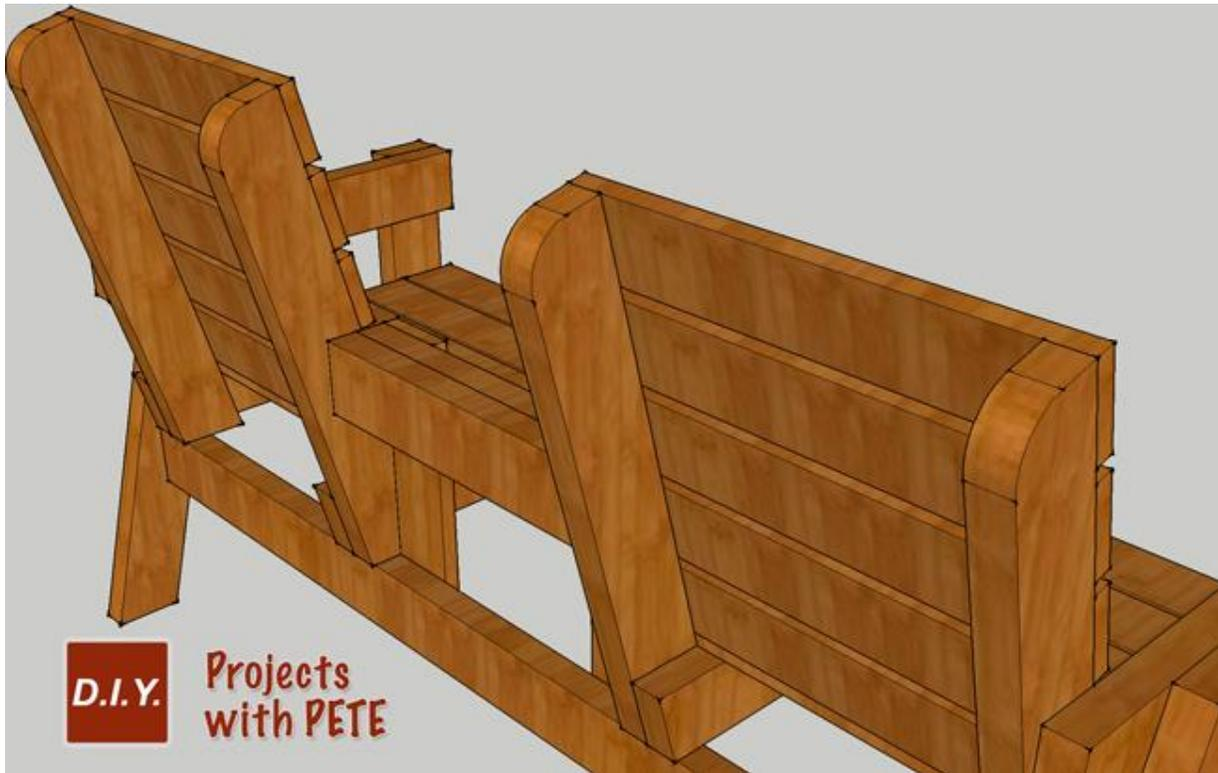
Attach the two middle backrest supports to the 17" 2×4 table support. This will strengthen the entire piece of furniture. Use two 3" deck screws on each side.
